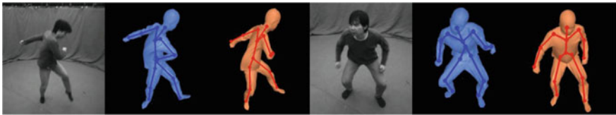
Fig. 5.6 Comparison with multi-view video-based tracking (MVT) approach on the “jump” sequence. The left three and the right three are input image, result of MVT, and result of the Kinect-based approach. On this fast motion, Kinect-based tracking succeeds, while MVT fails to capture the arm motion
